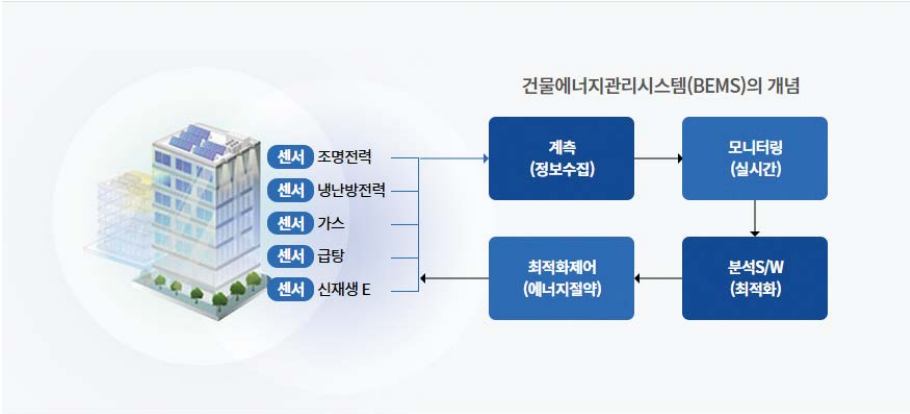
[Photo 4] Korea Energy Agency's BEMS (Building Energy Management System) Conceptual Diagram
